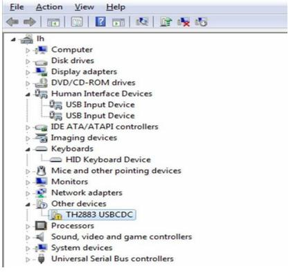
Figure 6-7 USBCDC has not been installed.
