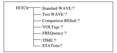
Figure 8-11 FETCh? subsystem command tree
