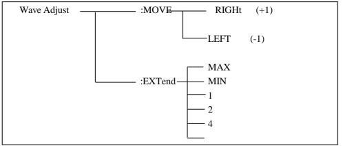
Wave Adjust subsystem commands
