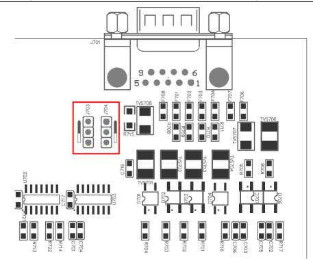
Figure 9-3 Jumper position on the Handler interface board
