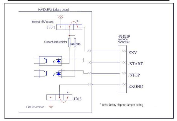
Figure 9-2 Simplified diagram of the input signal
