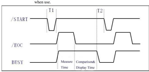
The timing diagram for handler interface is displayed in above figure, T1 is the trigger pulse width and the minimum pulse width is 1 us. T2 is the delay time, after the foregoing measurement completed to next trigger signal; its minimum pulse width is 0 us. /PASS and /FAIL signals are asserted after the measurement completed, till next trigger. The request of the /STOP pulse signal is the same as /START pulse signal.
