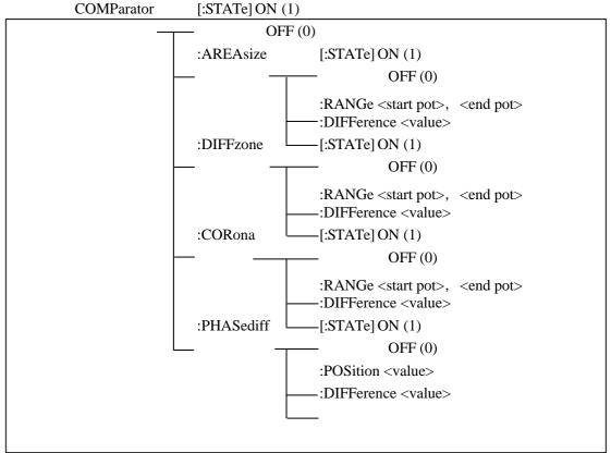
Figure 8-5 COMParator subsystem command tree
