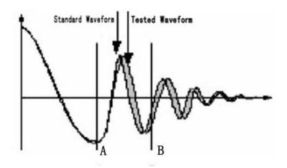
Figure 2-2 Differential Area Comparison
