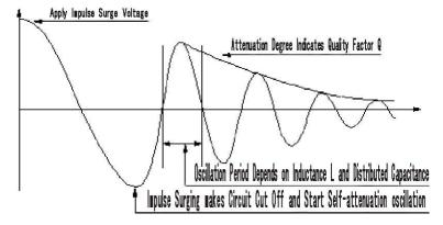
Figure 1-2 Typical self-attenuation oscillation wave
