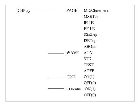
Figure 8-3 DISPlay subsystem command tree
